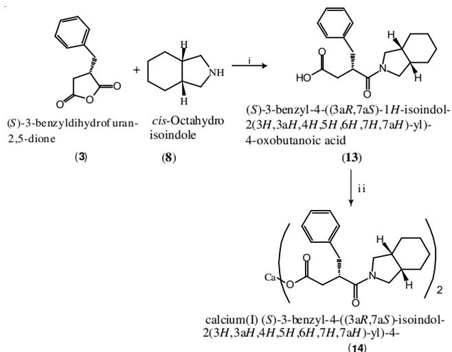
**Scheme-VI:** Reagents and conditions (i) Toluene, 40-45 °C (ii) NaOH, H<sub>2</sub>O, calcium chloride, ethanol, 25-30 °C
