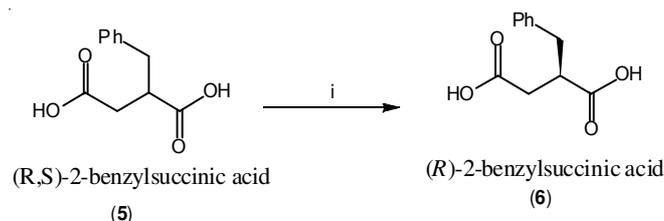
**Scheme-II:** Reagents and conditions: (i) (S)- $\alpha$ -Methylbenzylamine, ethanol, Dichloromethane, Conc HCl 25-30 °C
