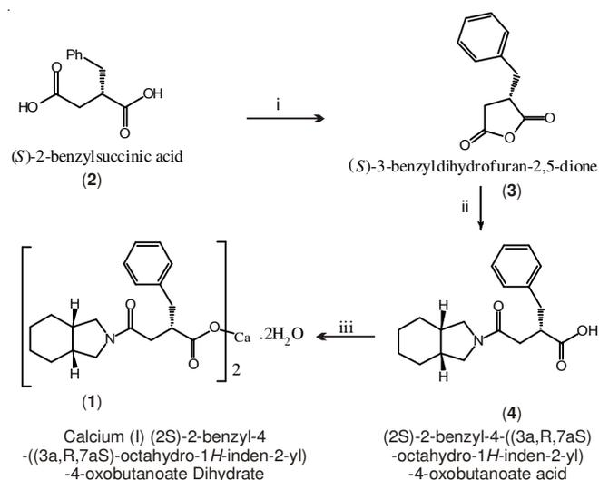
**Scheme-I:** Reagents and conditions: (i) Dichloromethane, acetic anhydride, 40-45 °C; (ii) *cis*-Octahydroisoindole, toluene, 40-45 °C; (iii) NaOH, H<sub>2</sub>O, calcium chloride, ethanol
