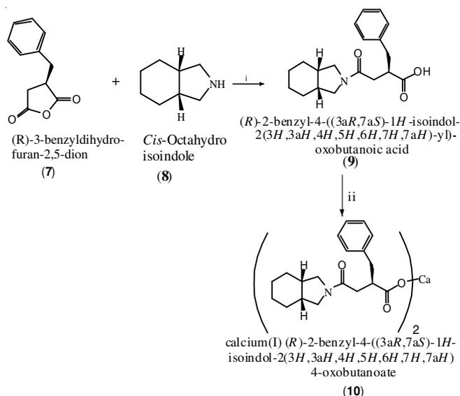
**Scheme-IV:** Reagents and conditions: (i) Toluene, 40-45 °C (ii) NaOH, H<sub>2</sub>O, calcium chloride, ethanol, 25-30 °C
