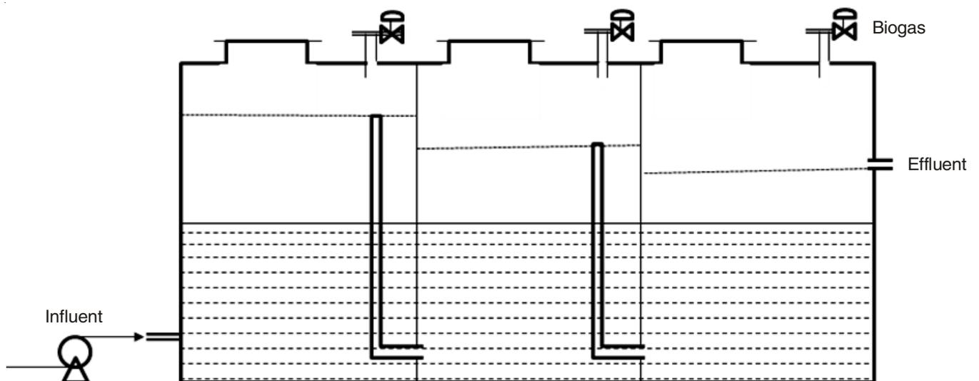
Fig. 3. Schematic diagram for anaerobic baffled reactor [Ref. 12]
