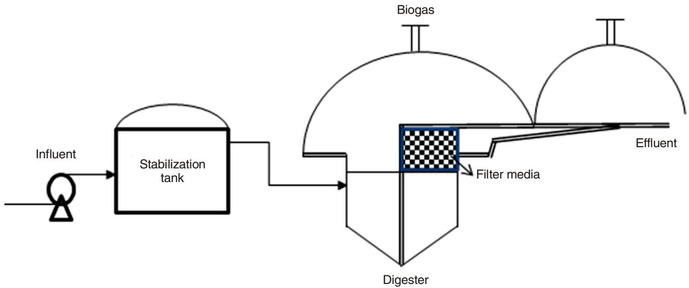
Fig. 1. Schematic diagram for fixed dome reactor [Ref. 12]
