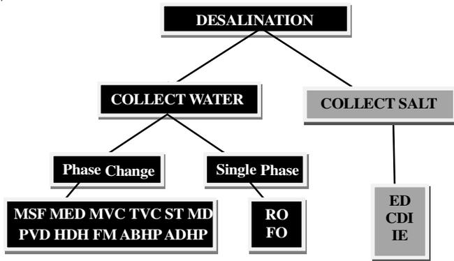
Fig. 3. Classification of desalination process [Ref. 10]
