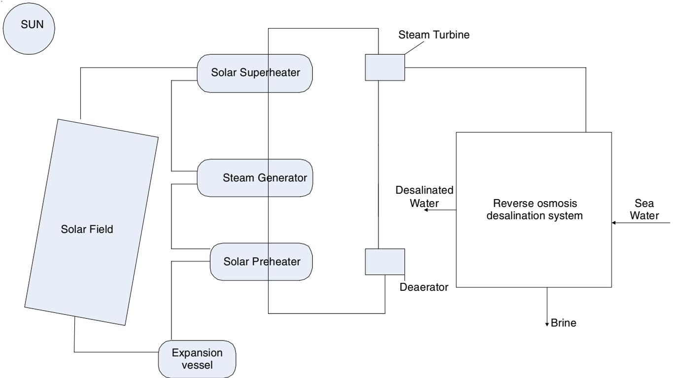
Fig. 9. Parabolic trough coupled with seawater reverse osmosis desalination unit [Ref. 4]
