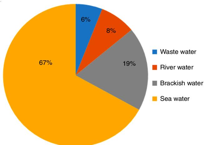
Fig. 2. Worldwide feed-water percentage used in desalination [Ref. 4]
