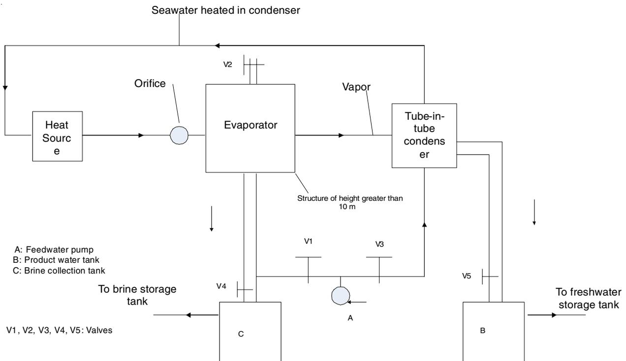
Fig. 4. Single-stage flash desalination system [Ref. 8]
