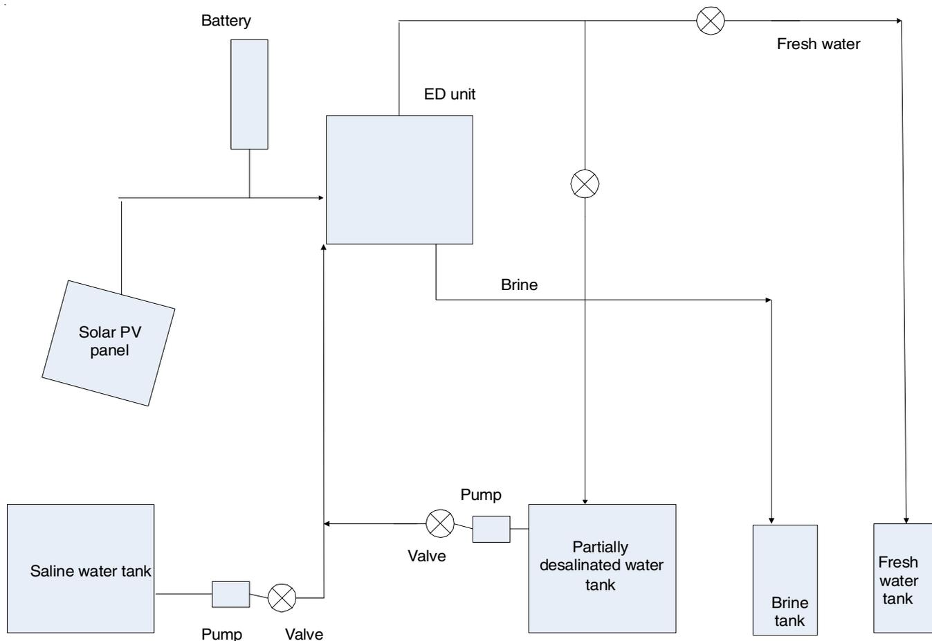
Fig. 8. Solar PV powered ED unit [Ref. 7]
