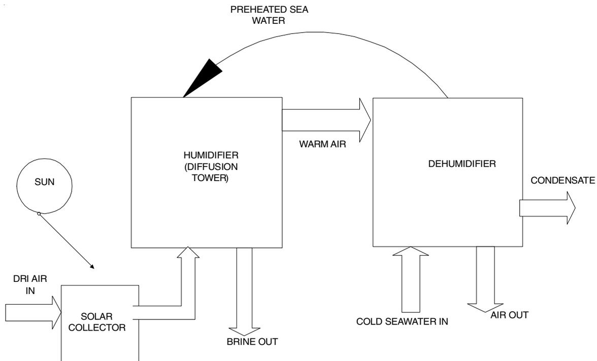
Fig. 7. A simple humidification–dehumidification (HDH) process [Ref. 16]
