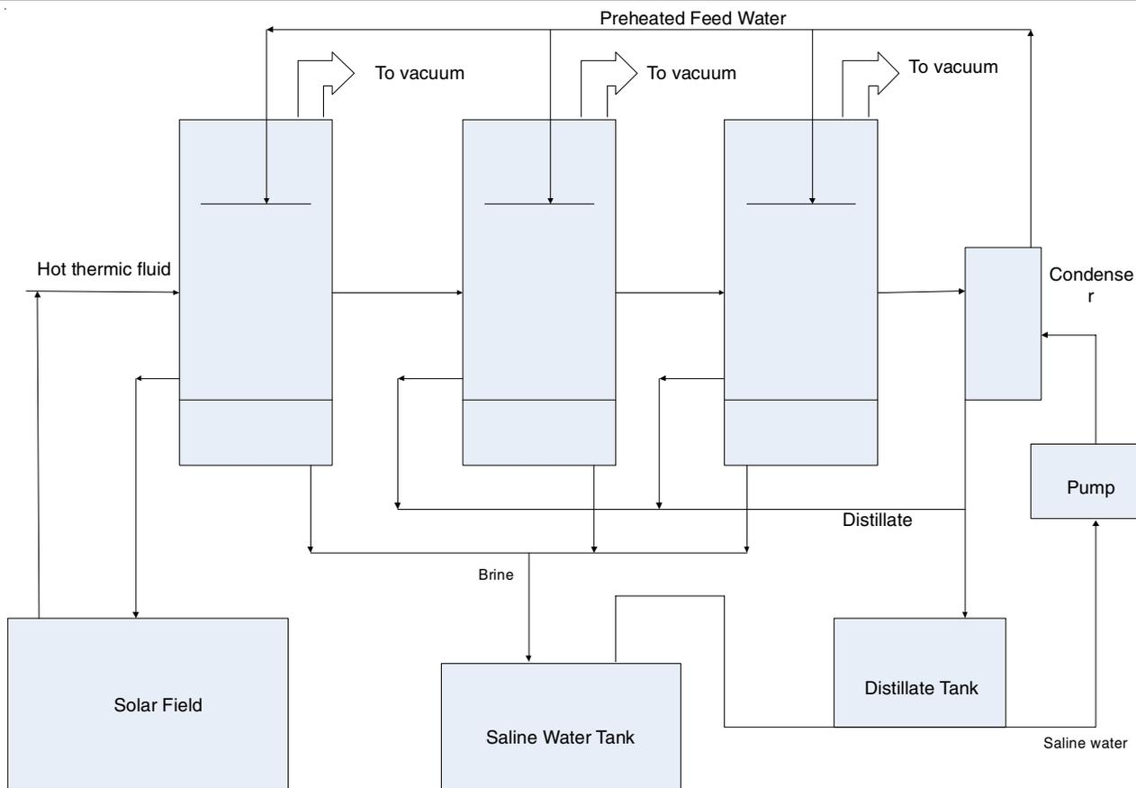
Fig. 5. Solar powered multi-effect distillation system [Ref. 7]
