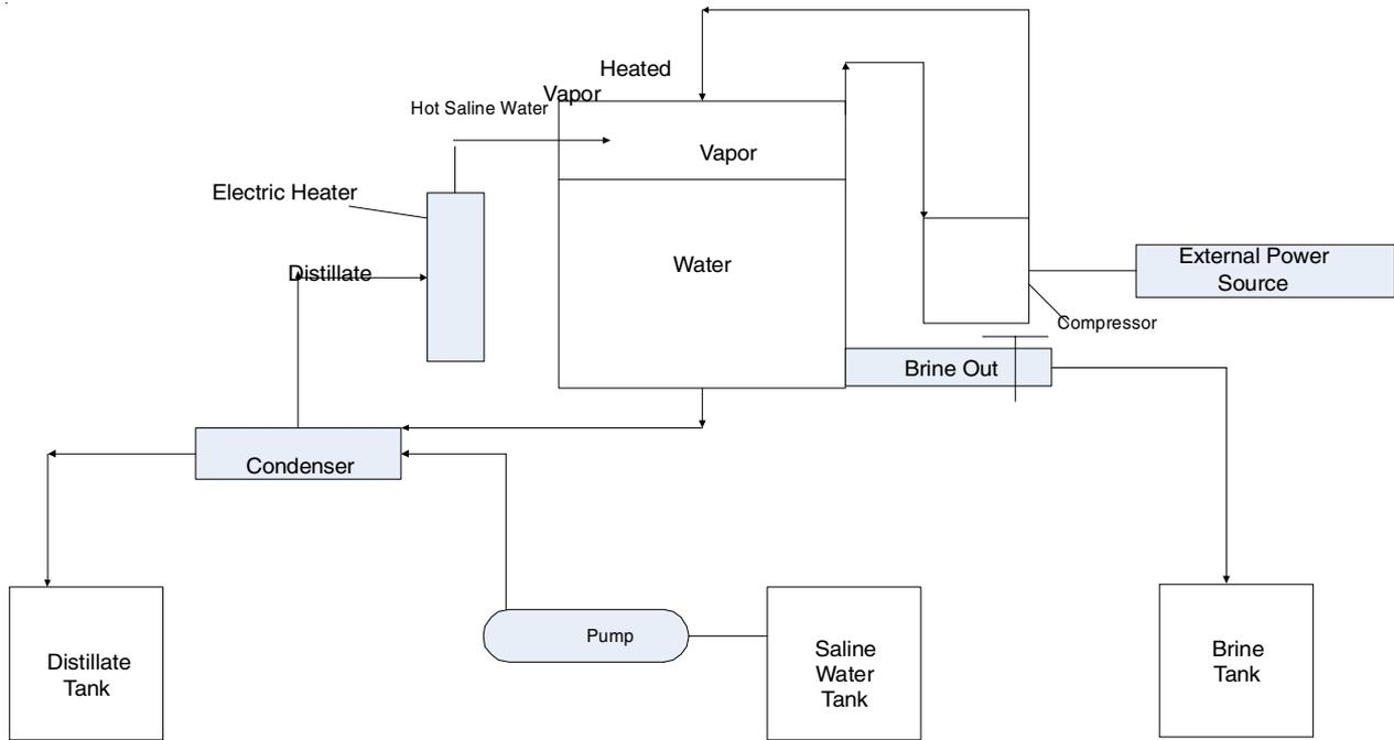
Fig. 6. Mechanical vapor compression desalination system [Ref. 7]
