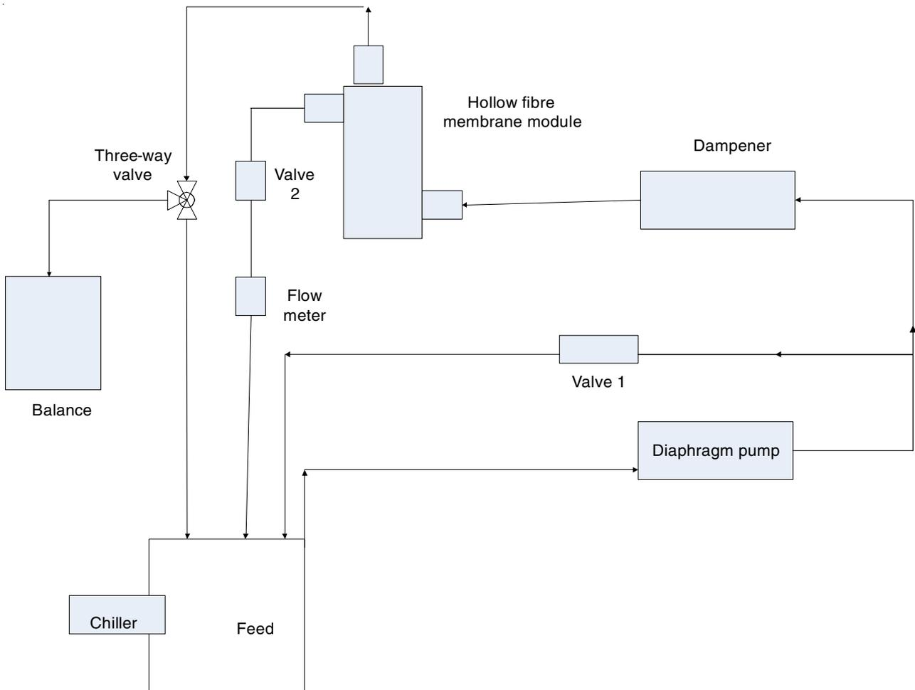
Fig. 10. Schematic diagram of the experimental nanofiltration set-up [Ref. 21]
